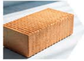
Wirecut Red Bricks – 9" Thick Outer Walls /4'6" Thick Inner Partition Walls
