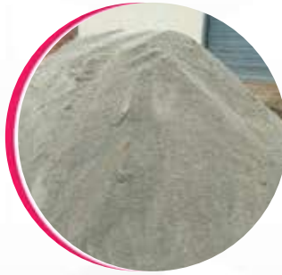
P-Sand For Plastering Works.
